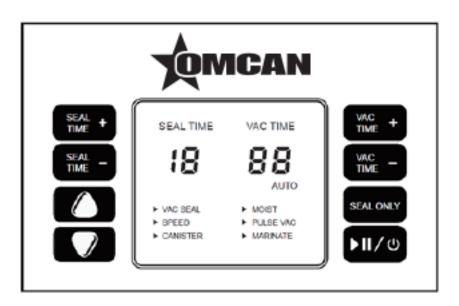
**Seal time +:** Button to increase the sealing time.
